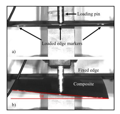
Figure 2 Bend-twist composite cantilever test setup. a) unloaded plate b) loaded plate.
