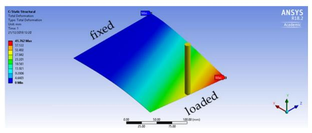
Figure 1 Finite element simulation of a cantilever bend-twist coupled composite under bending load. Total deformation plotted.
