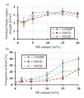
Fig. 1 Charpy impact strength a) and elongation at break b) of PLA/NR blend at different D-lactide content
