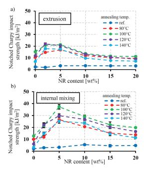
Fig. 8 Notched Charpy impact strength of annealed PLA/NR blends produced by extrusion a) and internal mixing b)
