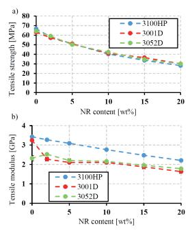
Fig. 2 Tensile strength a) and tensile modulus b) of different PLA/NR blends at different D-lactide content
