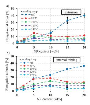
Fig. 9 Elongation at break of annealed PLA/NR blends produced by extrusion a) and internal mixing b)
