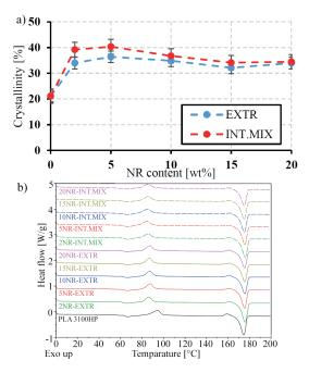
Fig. 6 Crystallinity a) and DSC first heating scans b) of PLA/NR blends produced by different techniques
