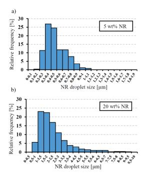
Fig. 5 Particle size distribution PLA/NR blends made with internal mixing at 5 wt% a) and 20 wt% b)
