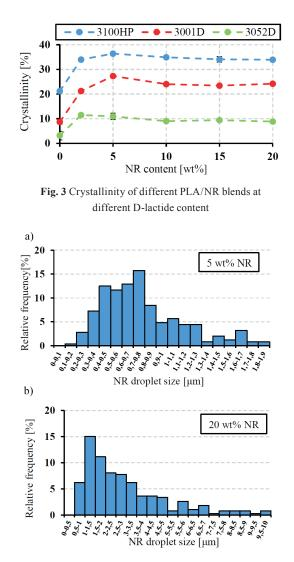
Fig. 4 Particle size distribution PLA/NR blends made with twin srew extrusion at 5 wt% a) and 20 wt% b)
