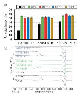
Fig. 7 Crystallinity a) and DSC first heating scans b) of annealed PLA/5NR blends produced by different techniques
