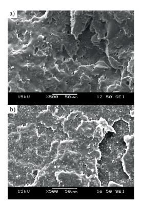
Fig. 10 SEM images of annealed PLA/5NR blends produced by extrusion a) and internal mixing b)
