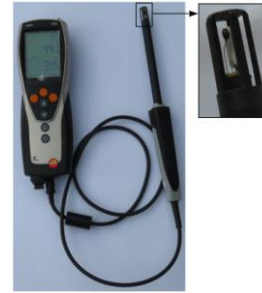
Fig. 5: The complex measuring instrument Testo-623 with data logger.
