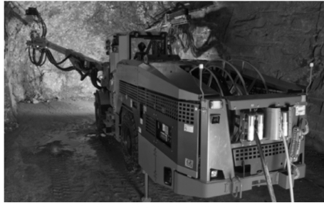
Fig. 1. SANDVIK DD421 robot manipulator [10] (with permission)
