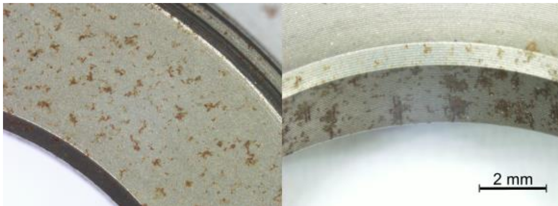
Figure 2. Corrosion patches before the operational
