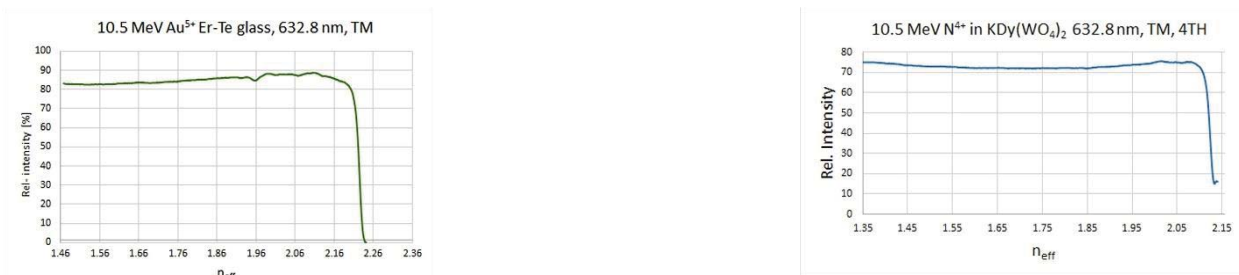
FIGURE 5. M-line spectra at 633 nm in TM mode a) of the 12.5 MeV Au 5+ irradiated Er-doped Te-W-glass. b) of the 10.5 MeV N 4+ irradiated KDy (WO 4 ) 2 crystal.
