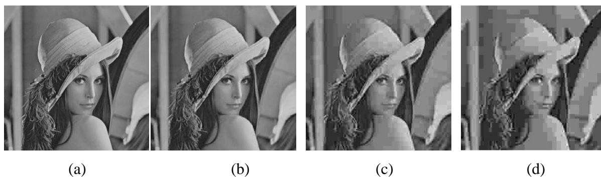
Fig. 1. Test image Lena with different compression ratios. (a) Original Lena image, Size: 64kB, bitrate: 8bpp, (b) Lena test image compressed with compression ratio 11, Size: 5.8kB, bitrate: 0.73bpp, (c) Lena test image compressed with compression ratio 30, Size: 2.1kB, bitrate: 0.27bpp, (d) test image Lena compressed with compression ratio 46. Size: 1.4kB, bitrate: 0.17bpp.
