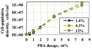
Figure 5. The cell-population density of samples as a function of foaming agent content
