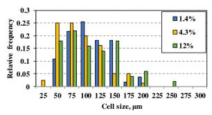
Figure 7. The cell size distribution of the foamed sample (2 wt% of syntactic foaming agent)
