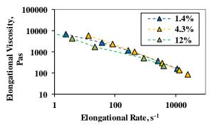
Figure 1. Elongational viscosity of PLA resins at 190 °C.
