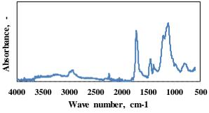
Figure 2. FTIR spectra of Tracel G 6800 shell material
