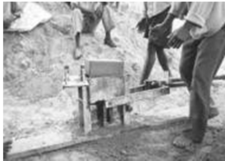
Fig. 4. The piston Sinfa used in mixing the components
