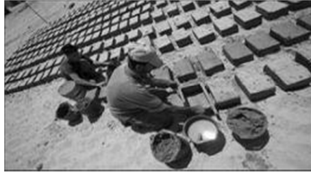
Fig. 3. Sand, water is the raw material to build a house in a way sandstone adobe
