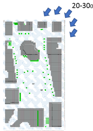
Fig. 1. The optimum street orientation for natural ventilation and outdoor thermal comfort
