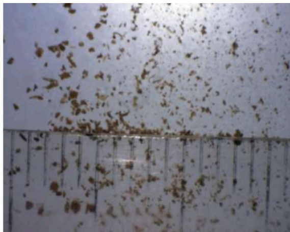
Figure 3. Corn leaf and stover in IL before pre-treatment (scale in mm is shown below the picture).
