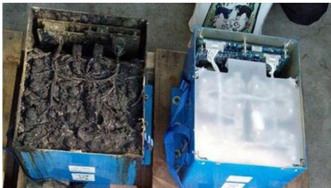
Figure 1. Fire of the Li-ion battery [3]
