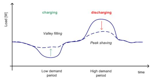
Figure 1. Valley filling and peak shaving with charging and discharging energy storage elements
