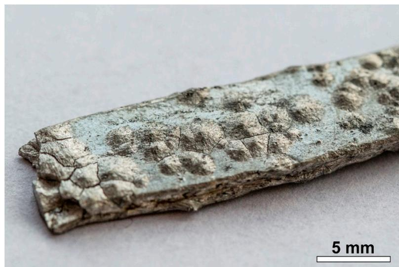
**Figure 1.** Tin pest warts and cracks on the surface of a tin solder bar; decomposition has already started at the ends of the bar.
