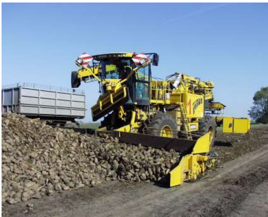
Fig. 2. Cleaning and loading machine in operation
