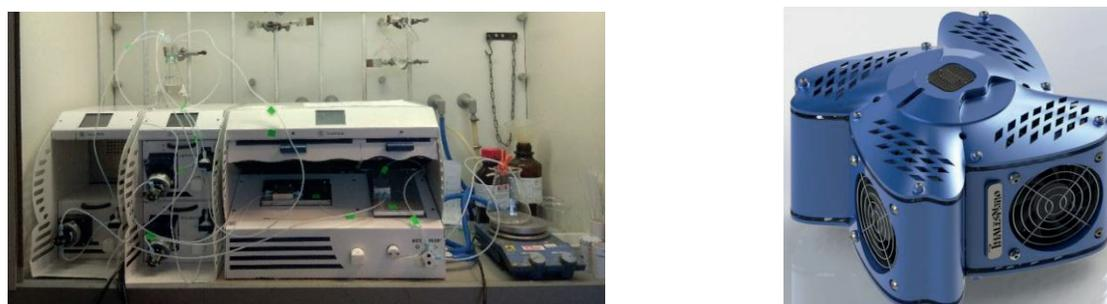
**Figure 30.** ThalesNano IceCube and PhotoCube reactor
