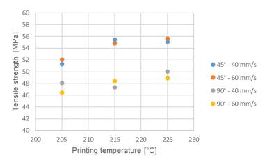
Figure 4. Tensile strength as a function of printing settings
