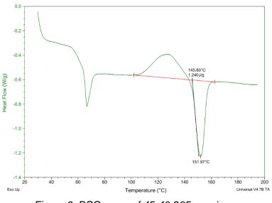
Figure 6. DSC curve of 45-40-205 specimen
