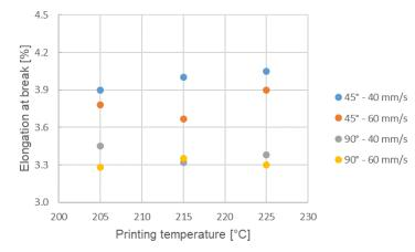
Figure 5. Elongation at break as a function of printing settings
