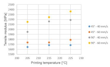
Figure 3. Tensile modulus as a function of printing settings
