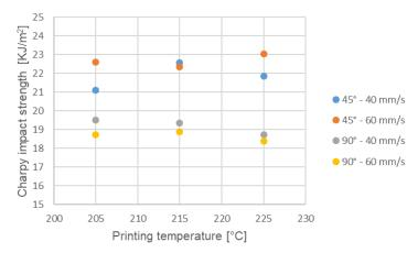
Figure 2. Impact strength as a function of printing settings
