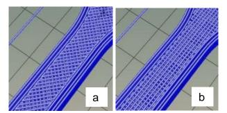
Figure 1. Printing structures, a: 45° orientation, b: 90° orientation
