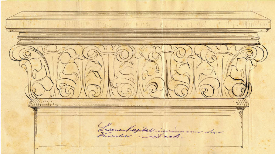
The drawing by stone-cutter Karl Kern to the capitals of the pillars. Source: Pannonhalmi Főapátsági Levéltár, unregistered documents of Kelemen Krizosztom, Restoration of the Deáki church and parish 1872–1875, 28.c.
