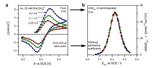
There are two links connecting the two methods: one is the experimental method of dynamic EIS (dEIS), and the other is a theoretical one: the potential program invariant (PPI) representation of the measured j(t) vs E(t) voltammetry data.
