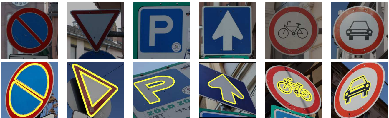
Fig. 6. Homography registration results on traffic signs. The first row shows the templates while below them the corresponding observations with the overlaid contour of the registration results.
