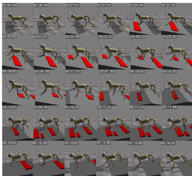
Fig. 15. Time-series snapshot of the simulated robot performance in slope terrain with sudden obstacles given. The detailed robot performance can be seen in the supplementary video.
