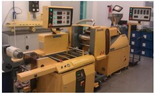
Figure 1. PLA film extrusion
