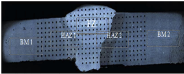
Fig. 2. Pipe after cutting and specimen after hardness measurement
