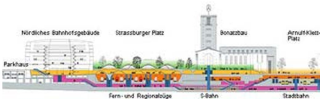
**Figure 7. - Vertical section of railway station plan, Stuttgart, Germany**
