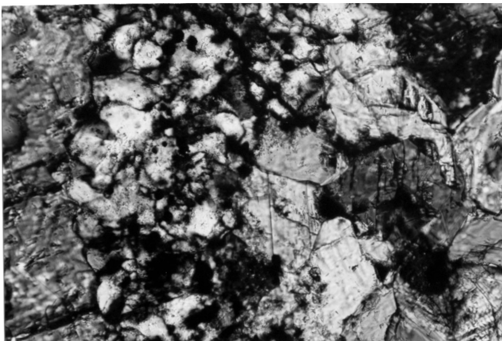
Pict. 6 Calcite rimmed by mosaic-textured quartz with pyrite dissemination. R 372-85m, andesitic tuff. Transmitted light, +N, 200x
