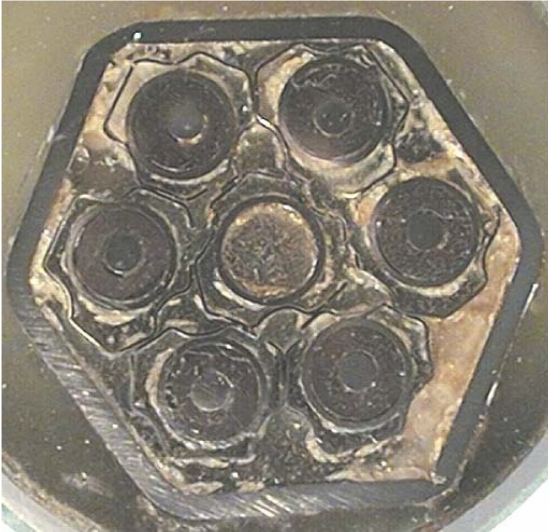
Fig. 33 CODEX-2 bundle cross section at 305 mm elevation
