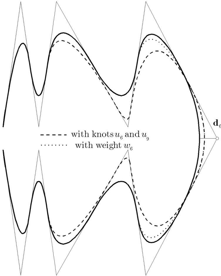
Figure 2: A comparison of two constrained shape modifications gained by the modification of two knots, and by the alteration of a weight ( $n = 12, k = 3, i = 6$ ).
