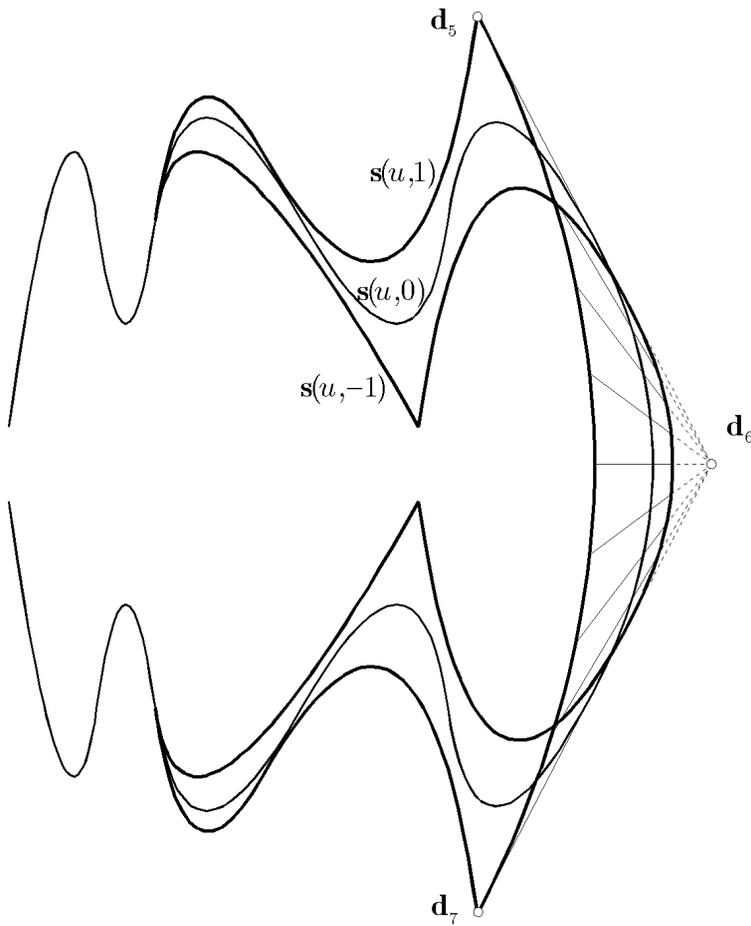
Figure 1: The effect of the symmetric modification of knots  $u_i$  and  $u_{i+3}$  on the shape of a quadratic B-spline curve, with the indication of paths of the arc  $s_{i+1}(u)$  ( $n = 12, k = 3, i = 6, \lambda \in [-1, 1]$ ).
