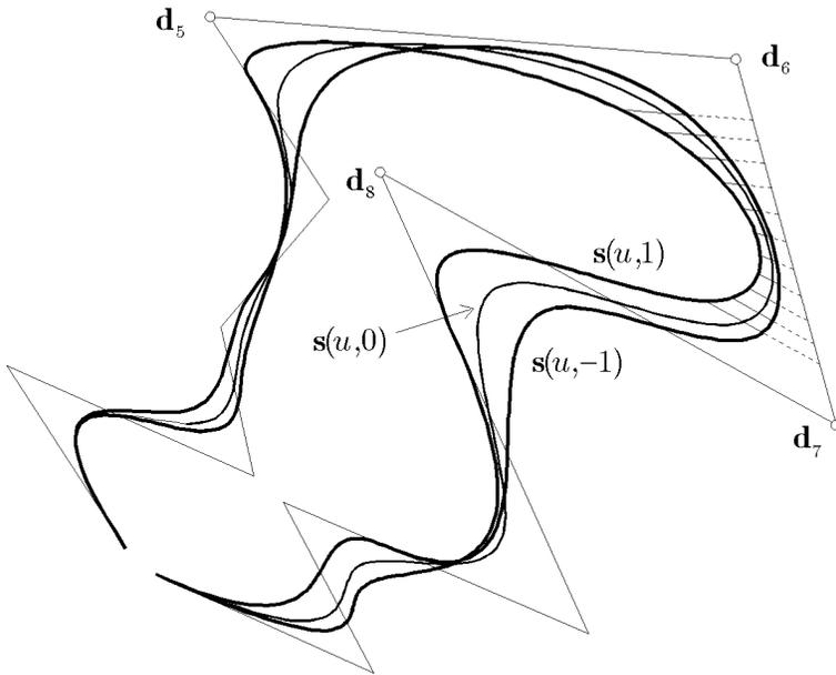
Figure 3: Shape modification of a cubic B-spline curve by means of a symmetric translation of knots  $u_i$  and  $u_{i+5}$ . Paths of points of the arc  $\mathbf{s}_{i+2}(u)$  are also shown along with their extensions which intersect the side  $\mathbf{d}_6, \mathbf{d}_7$  of the control polygon ( $n = 12, k = 4, i = 6, \lambda \in [-1, 1]$ ).
