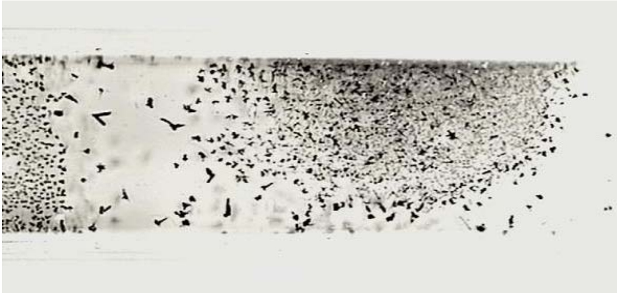
Fig. 9. RuO 2 crystals precipitated in the gas flow and deposited on the inner surface of a quartz sampler tube.
