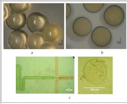
*Figure 1 Images of microspheres (a), microcapsules (b), and microparticles prepared by microfluidics (c)*
