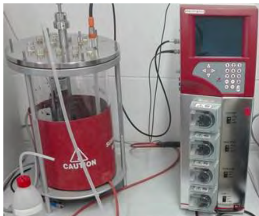
Figure 1. Units of Fermac 320
