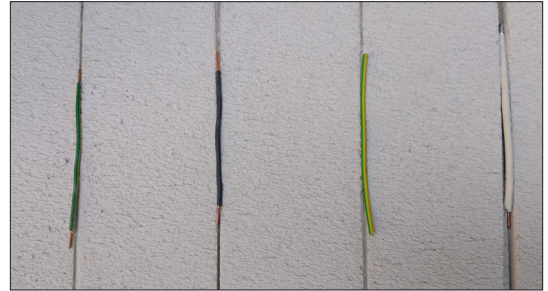
Figure 2. Concrete brick prepared with copper cables
