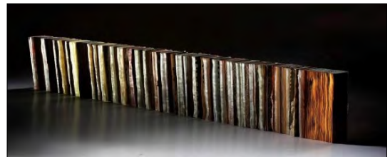
Figure 3. Composite prototype of straight noise protection wall: materials: wood, porcelain, ceramics, glass [2]
