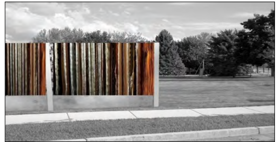
Figure 2. Three-dimensional model of noise-shielding wall: base material: wood, porcelain, ceramic, glass [2]
