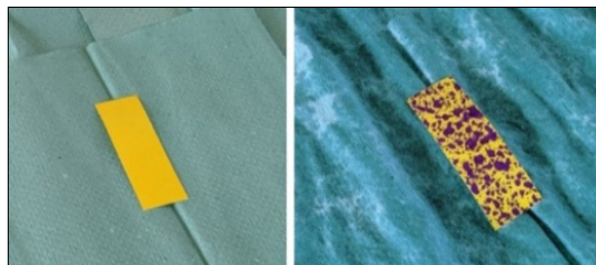
Figure 6. Water-sensitive paper before and after treatment
