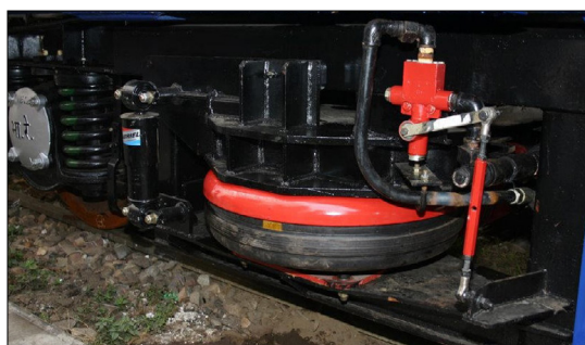
Figure 1. A bogie of a railway vehicle assembled with a spiral and a belted air spring. [1]
