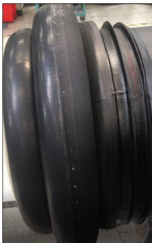
Figure 11. Backfolding with bellow.
