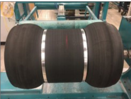
Figure 4. Folding back the edge of the carcass.
