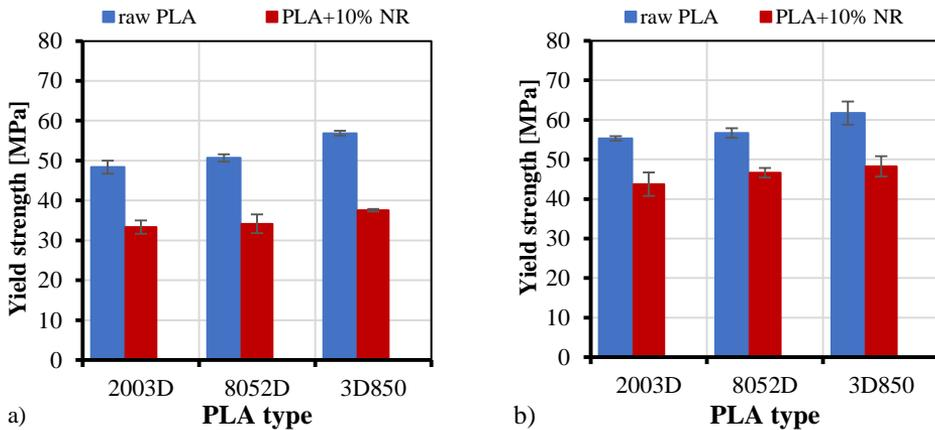
Figure 2. Yield strength of the fabricated samples with (a) grid-type infill pattern and (b) unidirectional infill pattern parallel to the length of the specimens
