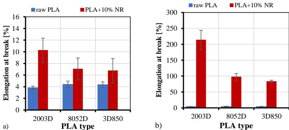
Figure 4. Elongation at break values of the fabricated samples with (a) grid-type infill pattern and (b) unidirectional infill pattern parallel to the length of the specimens
