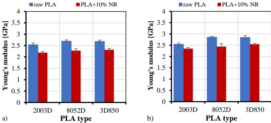
Figure 3. Young's modulus of the fabricated samples with (a) grid-type infill pattern and (b) unidirectional infill pattern parallel to the length of the specimens
