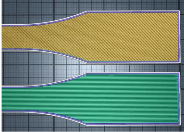
Figure 1. Schematic graphic of the printing orientation with respect to the specimen
