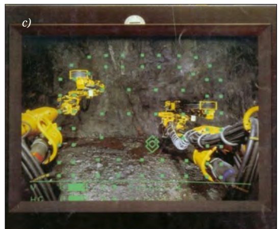
Figure 6. The prescribed drilling scheme (a), the boom with the conductive rail (b), the display screen (c).
