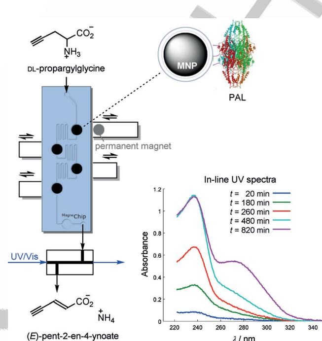
**Figure 1.** Ammonia elimination from *D,L*-propargylglycine in a light-protected microfluidic reactor with multiple magnetic cells filled with PAL immobilized on MNPs and equipped with an in-line UV/Vis detector (reaction in  $D_2O$  at pH 8.8,  $37^\circ C$ ). The progress of the reaction was followed in the full UV spectra.
