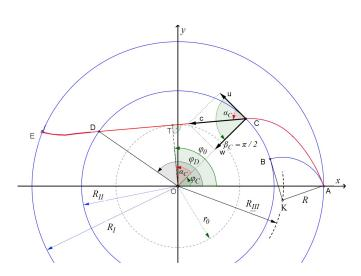
Figure 5. The shape of an absolute streamline in the runner
