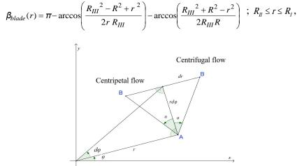
Figure 4. The relationship between the directional angle  $\alpha$  of the absolute velocity and the elementary triangle defined by the differentials
