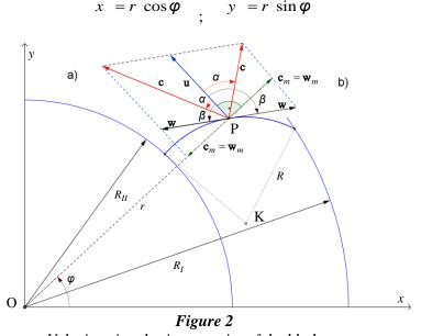
Velocity triangles in one point of the blade curve a) along the centripetal section b) along the centrifugal section
