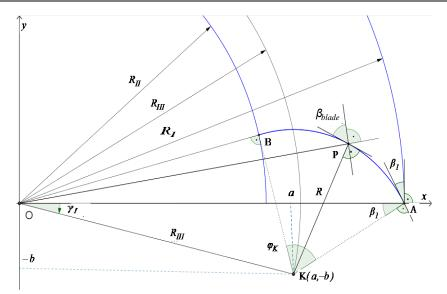
Figure 3. Geometry of a circular blade arc
