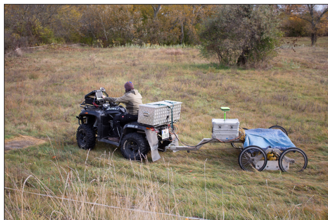
Fig. 4. Experts of the Ludwig Boltzmann Institute carry out a magnetometer survey at the site of the former Matrica auxiliary camp in Százhalombatta. Photo by Zsuzsanna Emília Kiss / BME, 2021
