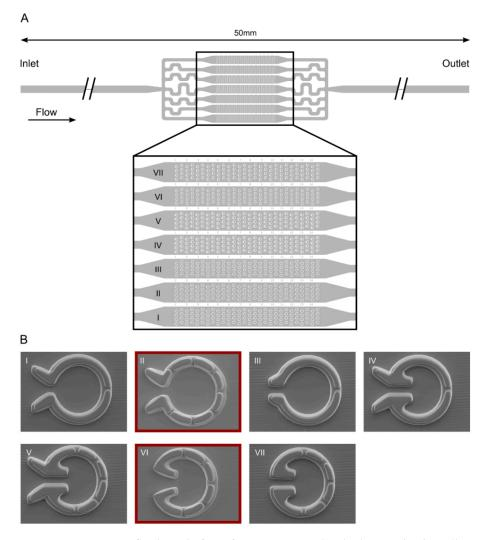
**Figure 3.** "Pot" microfluidics platform for capturing individual *C. reinhardtii* cells enabling cell division and the measurement of their photosynthetic activity. (**A**) Scheme of the device with seven different types of traps located in parallel channels. (**B**) Scanning electron microscopy images of the individual traps.
