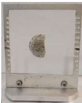
Figure 1. A cut from the cement cylinder (250 OXY-B) and its sample support used to gather localized boron profile from the PGAI measurements. The scan was accomplished along the vertical diameter of the sample. Photograph courtesy of Zoltan Kis.
