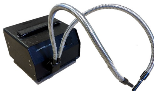
Figure 2. BEL Halogen illuminator used for in-line real-time image analysis in the final continuous crystallization experimental setup.
