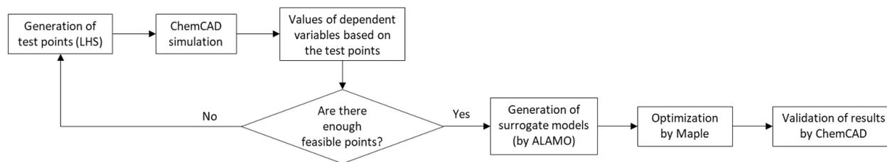
**Fig. 1** Flow chart of the surrogate model-based optimisation method.
