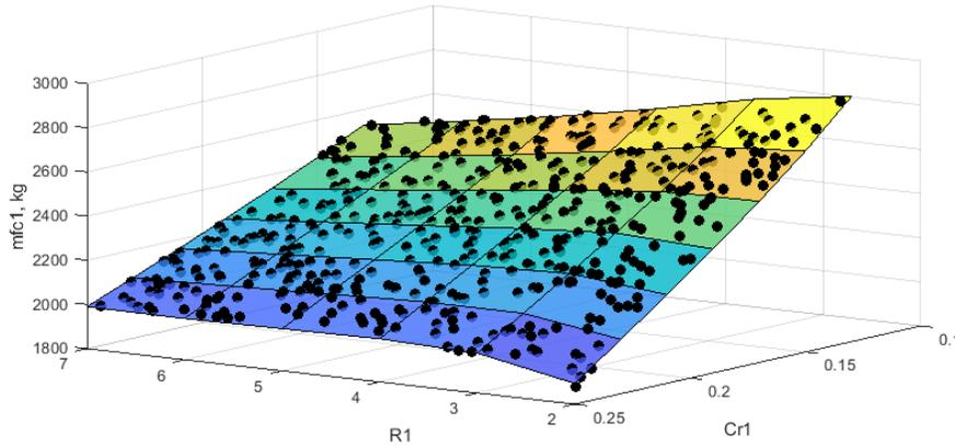
**Fig. 2** Mass of Fore-cut 1 calculated by simulation (dots) and by the surrogate model fitted (surface).
