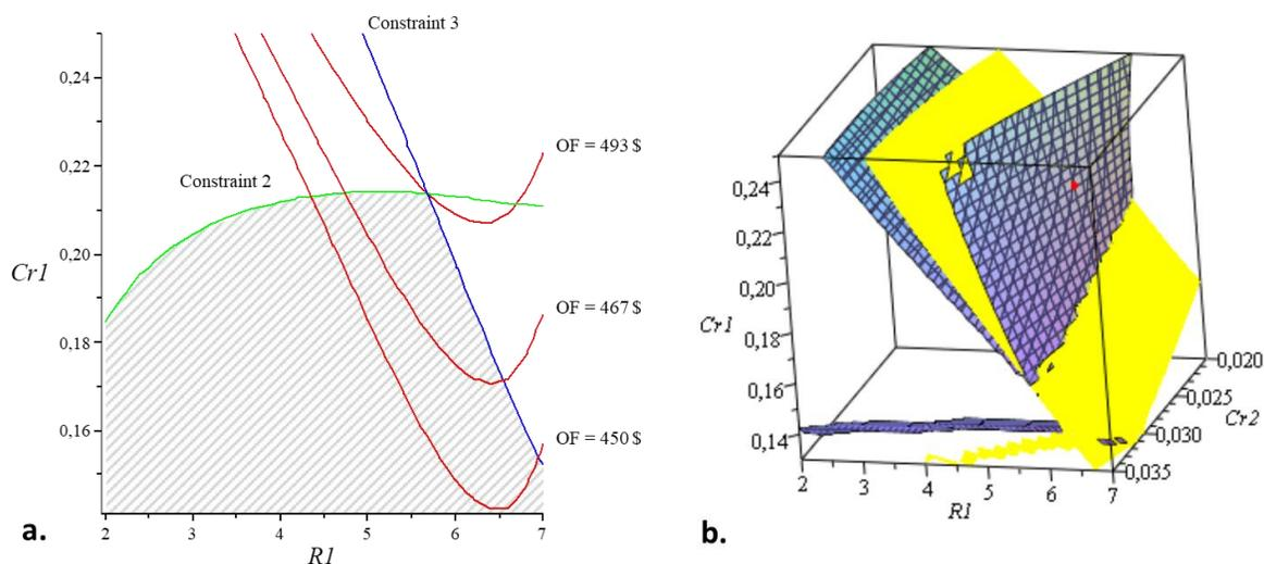
**Fig. 3** a. Contour plot of OF (red lines) with  $R_1$  and  $Cr_1$  as independent variables. Constraint 2 is shown as a green line, Constraint 3 as a blue one, b. plot of the active constraints (multicolour surfaces), the limit of surrogate model validity (yellow surface) and the optimum obtained from the surrogate models (red dot).
