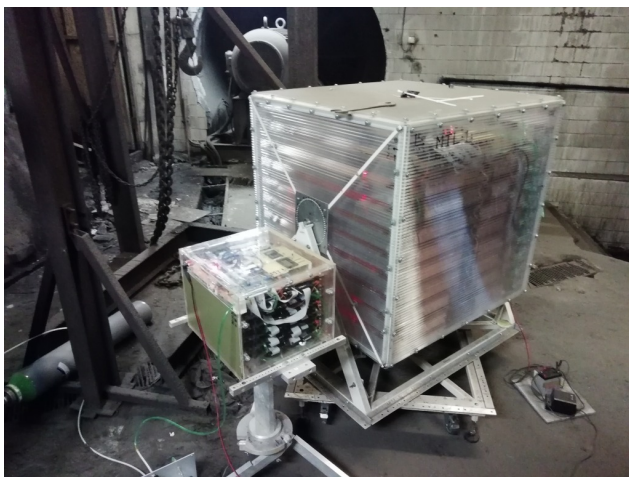
Figure 1. The Small (25 cm) and the Large (80 cm) Muograph next to each other in a tunnel below the Castle of Buda.
