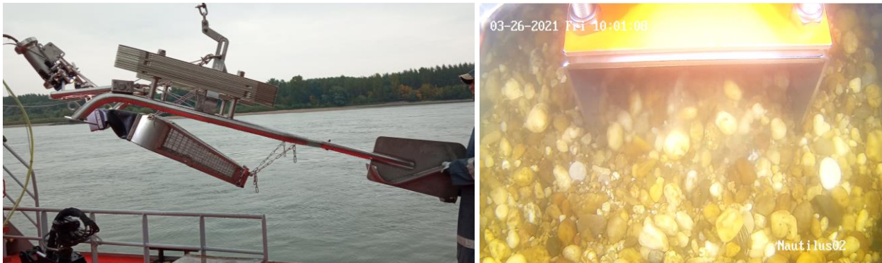
Fig. 1. BfG-type bedload sampler (left), video footage from the camera fixed to the sampler (right).
