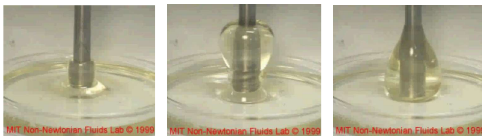
Fig. 2 Up climbing (left), relaxing on top (center) and down falling (right) phases of Weissenberg effect [8]
