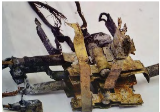
Figure 2. Galvanic corrosion affected damage
