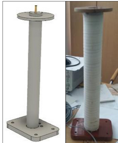
Figure 4. The 3D model (left) of the solenoid and the manufactured solenoid (right).
