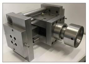
Figure 1. Proportionally reduced equipment for determining FLD.
