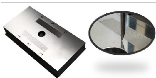
Figure 4. The marked measuring sections on the insert, used for contour measurement [3]
